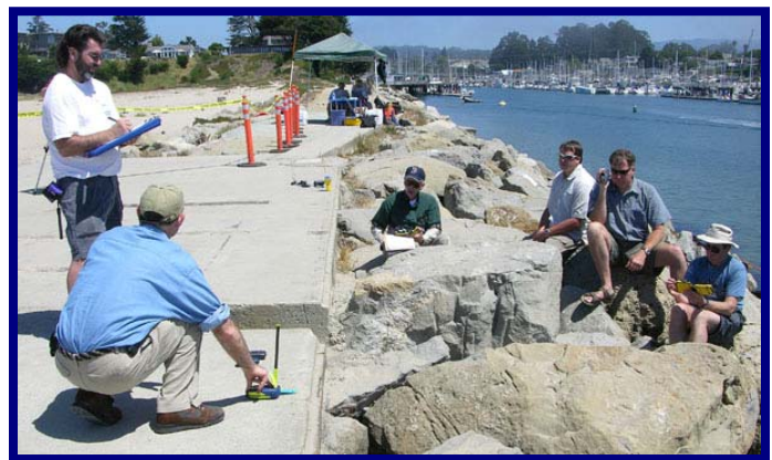
Baseline Scenario Alpha – Doug Ritter preparing to activate ACR PLB-200, manual recording of GPS location and time, WS Technologies BT100A receiver operators on rocks below.
