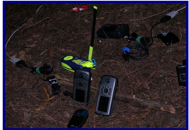
ACR Model PLB201 without GPS showing light colored faceplate
