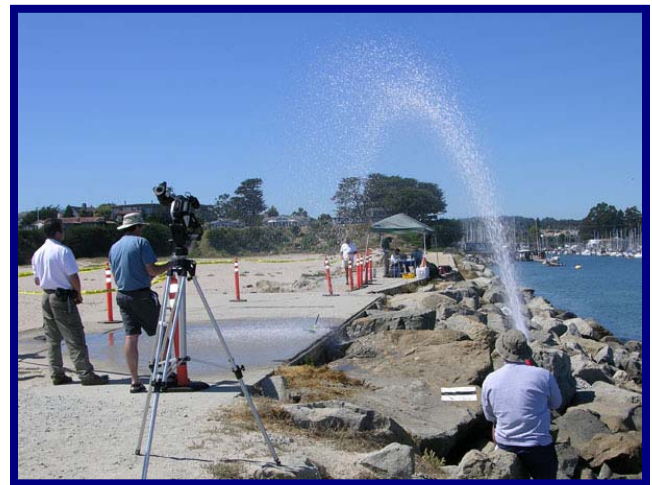
Baseline Scenario Charlie – Simulated rain on ACR Prototype PLB
