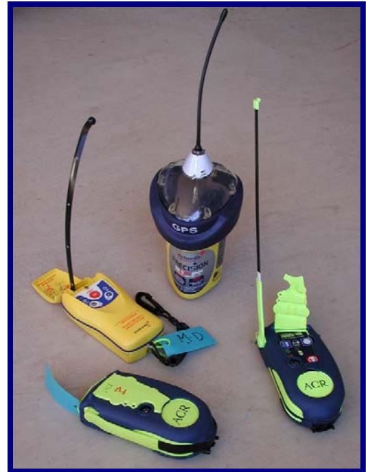
Location Protocol 406 MHz Emergency Beacons tested: (clockwise from 12:00) McMurdo Precision EPIRB, ACR, AquaFix PLB-200, ACR Prototype PLB, McMurdo Fastfind Plus PLB
