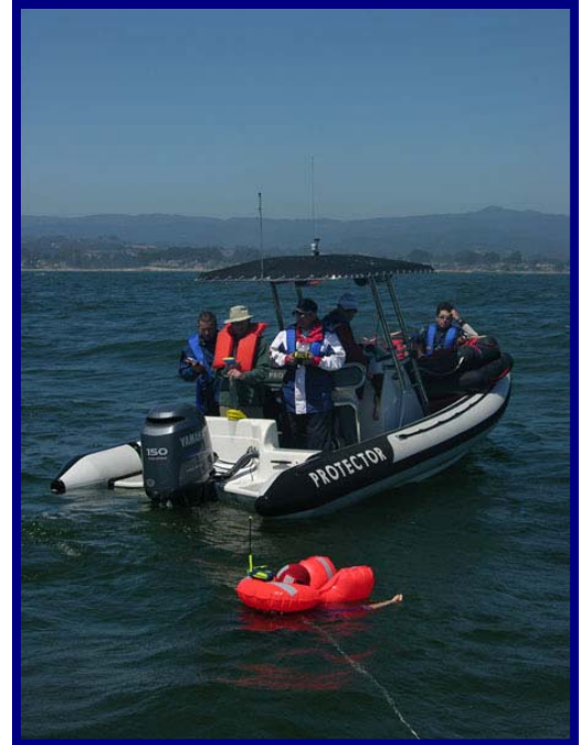
Maritime Scenario Golf – ACR Prototype PLB attached to PFD on Oscar with BT-100A test receivers in RIB.
