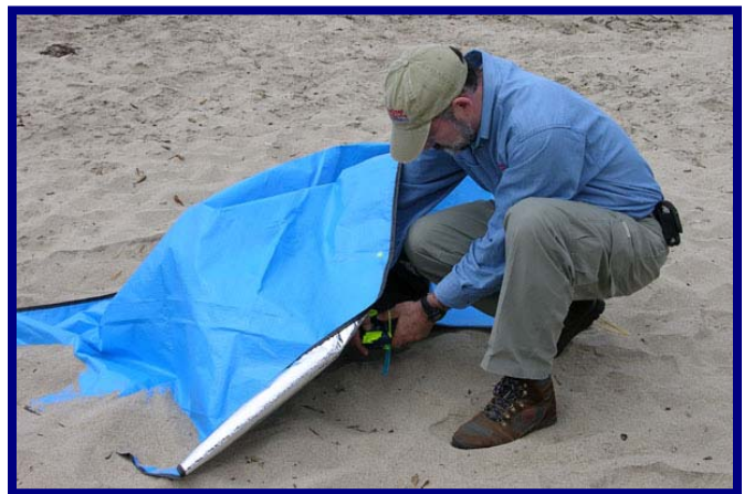
Inland Scenario Golf – Doug Ritter activating ACR PLB-200 under cover to prevent initial GPS acquisition
