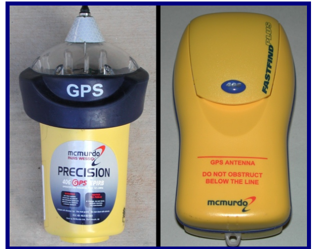
Upgraded McMurdo Location Protocol Beacons: Precision 406 GPS EPIRB (left), Fastfind Plus GPS PLB (right)
