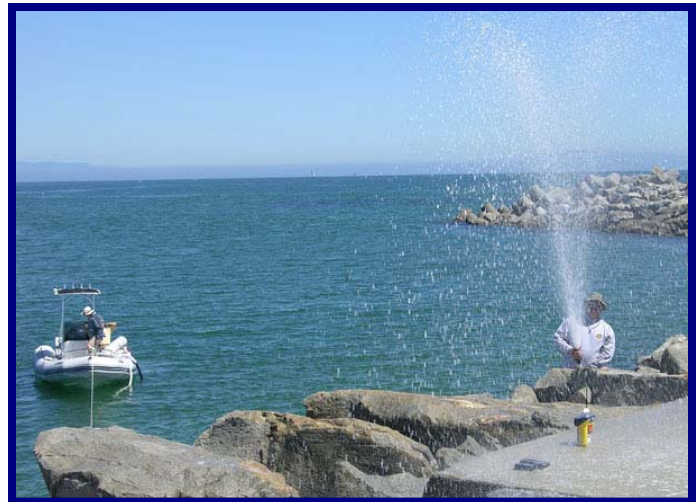
Baseline Scenario Charlie – McMurdo Precision EPIRB – RIB with fire pump and MCPO Flythe manning the hose creating simulated rain on the beacon.
